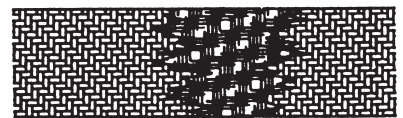
Figure 9 Other Apparent Damages That May Affect Strength Ratings; Such As Crushed Webbing, Etc.
